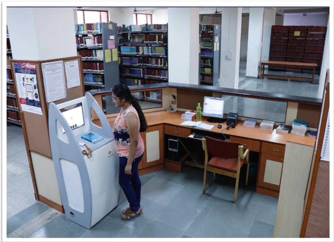
Fig 5: RFID Shelf Check-In & Check-Out (KIOSK) System
